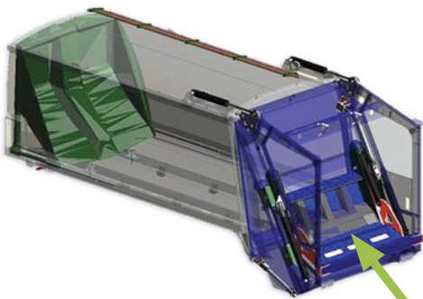
Packer plate shuts down when maximum load is reached
